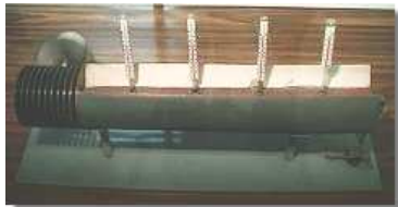
Experimental setup to measure classical heat conduction (Deutsches Museum München)
